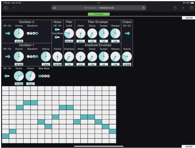
Fig. 2. The synthesiser interface running on an iPad touchscreen computer. This includes a representation of a typical synthesiser with a simple step sequencer for creating a loop of notes. The synth interface is available online at http://metatone.net/model-d/
